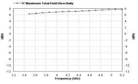
Fig: 16. Directivity Graph (showing total field directivity of 7.56 dBi at 4.9 GHz band) for Basic Rectangular Patch Antenna
