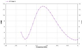
Fig: 22. VSWR (1.68 & 1.35 at 3.97 GHz & 4.96 GHz respectively) of Slotted Microstrip Rectangular Patch Antenna
