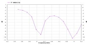
Fig: 12 Return Loss of Basic Rectangular Patch Antenna at Feed Point (6,-6)
