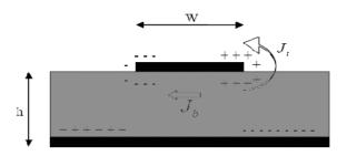
Fig: 8. Charge Distribution and Current Density Creation on the Microstrip Patch
