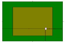
Fig: 11. Designed Basic Rectangular Patch Antenna Showing Feed Point (6,-6)
