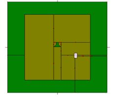
**Fig: 19.** Designed slotted rectangular patch antenna showing feed point (5,-3)
