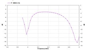
Fig: 21. Return Losses (-12.34dB & -16.46dB at 3.97 GHz & 4.96 GHz respectively) of Slotted Microstrip Rectangular Patch Antenna at Feed Point (5,-3)
