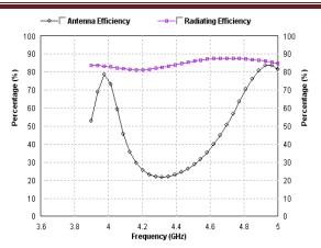
Fig: 23. Antenna and Radiating Efficiencies (antenna efficiency 83.35% & radiating efficiency 85.20% for the Second band) of Slotted Microstip Rectangular Patch Antenna
