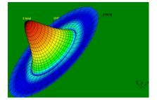
Fig: 14 Radiation pattern of Basic rectangular patch antenna at Feed point (6,-6)
