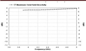
**Fig: 26** Directivity Graph (showing a directivity of 7.58 at 4.96 GHz) for Slotted Rectangular Patch Antenna
