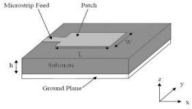
Fig: 5. Microstrip Patch Antennas
