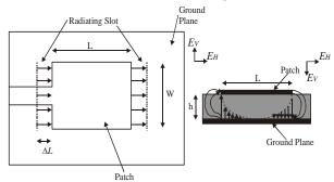
Fig: 6. Top View of Antenna, Fig: 7. Side View of antenna
