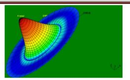
Fig: 20 Radiation Pattern of Slotted Microstrip Rectangular Patch Antenna at 4.96 GHz
