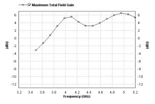
**Fig: 17.** Field gain Graph (showing total field gain of 6.45 dBi at 4.9 GHz band) for Basic Rectangular Patch Antenna
