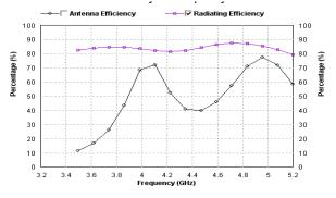
**Fig: 18.** Antenna & Radiation Efficiency Graph (showing antenna & radiating efficiencies of 77.21% & 84.9% at 4.9 GHz band) for Basic Rectangular Patch Antenna
